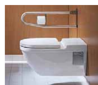
Accessible toilets With a seat height of 450 - 500 mm and a projection of 700 mm, barrier-free wall-mounted toilets in compliance with DIN 18040 enable ease of transfer and independent usage to the greatest possible extent.
